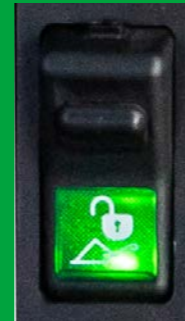
Safety Switch (loader)
