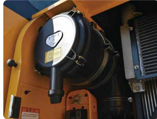
21T large capacity air filter reduces restriction of air inflow and enhances engine performance.
