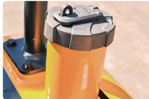
270L super large fuel tank and double-lock cover of fuel tank
